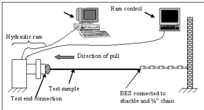
Figure 4. Break test set up in laboratory.
